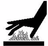
Warning: Hot surfaces.
