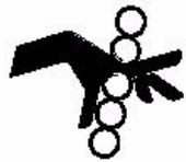
Warning: Pull-in hazard.
