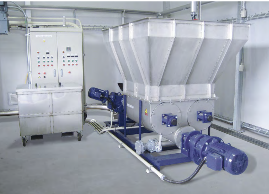
Pump of range BTEIM with two paddle shafts, special hopper design, enlarged cross section and conveying screw with integral knives in the compression zone handling food waste.
